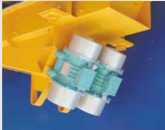
Trough conveyor to charge an elevator with up to 12 m 3 /h glass batch
