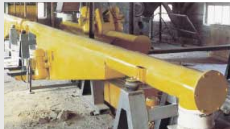
Enclosed conveying protects from unwanted contamination of the transported material and of the environment
