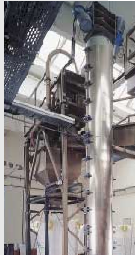
PVC granules must overcome large differences in height in a confined space of ground. Spiral conveyors offer the possibility of processing the conveyed material in addition to the transport function
