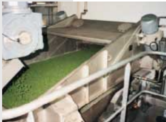
Trough and tubular conveyors and screens which are specially designed for the stringent hygiene standards of the foodstuffs industry are used for vegetable processing
